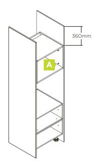
Attach the 600mm microwave box 360mm from the top of the end panels.
