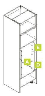
Attach both oven cleats 20mm back from the front of the end panels.
