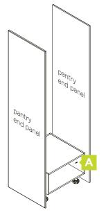
Set the drawer cabinet back from the front of the end panels 18mm for melamine doors and 20mm for thermoformed doors.
