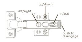
**c.** To align doors adjust marked screws.
