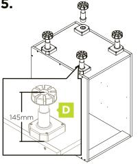
Set height of the adjustable feet to 145mm.
