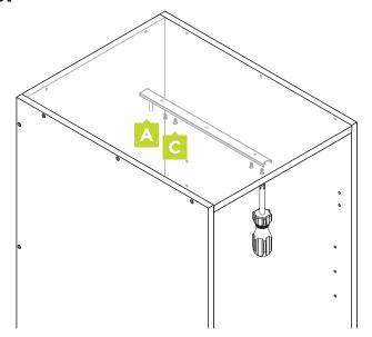
Carefully remove the guide from the top of the runner (A). Push the black plastic lever to the right to release the guide. Align the runner with the pre-drilled holes and fix to the cabinet using 2x18mm wood screws (C). Use an additional 2 screws for added strength.
