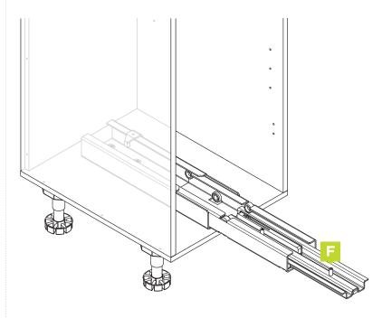
(ii) Reassemble the bottom runner. The soft close runner should operate smoothly if reassembled correctly.
