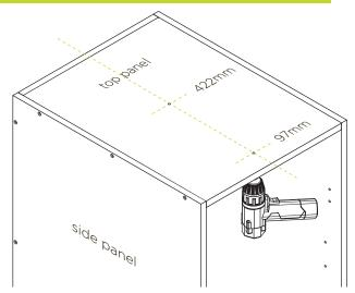
On the pantry top panel, draw a straight line down the centre and mark out holes to be pre-drilled at 97mm and 422mm from the front edge.
