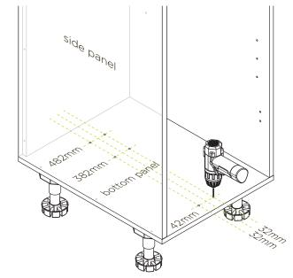
On the pantry bottom panel, draw a straight line down the centre and then draw parallel lines 32mm over on each side. Next mark out holes to be pre-drilled at 42mm, 382mm and 482mm from the front edge.
