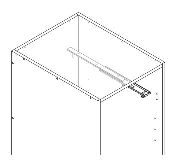
(i) Slide the guide back onto the runner. The runner should operate smoothly if reassembled correctly.
