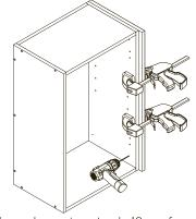
Pre-drill and attach using 28mm screws.
