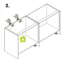
The back of the panel sits directly on the floor. Trimming may be necessary on a uneven floor.
