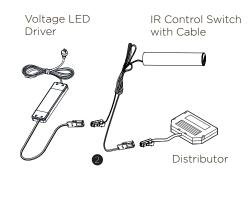
If you are using an **IR Control Switch** with the **75W Driver**, the Distributor cannot be separated.
