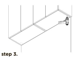
Using an 2.5mm drill bit pre-drill the marked out holes to a depth of 3mm
