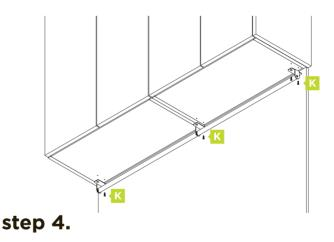
Align the assembled rail with the pre-drill holes and using the cabinet screws, fix the product to the cabinet.
