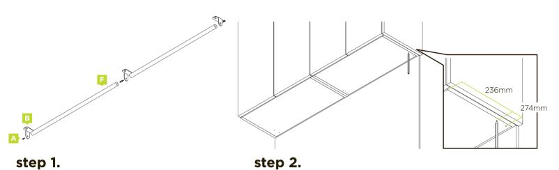
Use the two accessory screws to fix the wall brackets to the end of the rail.
