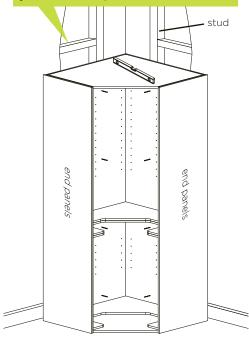
Ensure the cabinet is level before attaching to the wall in at least eight locations.
