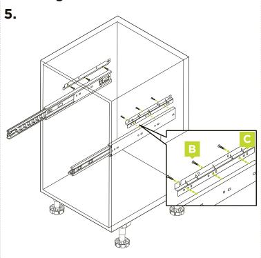
Using the top sets of pre-drilled holes, align with the 2nd, 5th and 7th holes on the lid brackets (C) and fix to the cabinet using  $6 \times 16$ mm wood screws (B) as pictured above.
