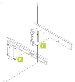
Position the door fixing brackets so the elongated holes on each bracket align with the holes drilled in Step 7. Ensure the open side of the brackets face inward as pictured above. Fix the brackets to the door using 4 x 14mm wood screws (F).
