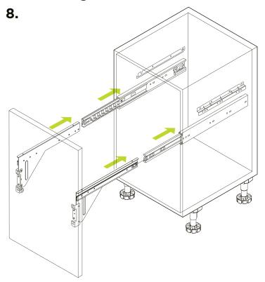
Carefully slide the guides back into the runners. The runners should open and close smoothly if assembled correctly. Extend the runners once they have been correctly reassembled.
