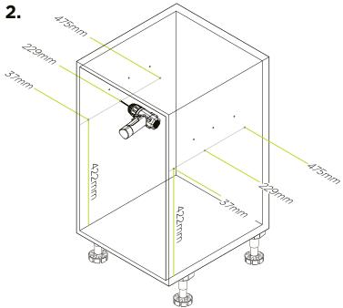
On both sides of your cabinet, draw a horizontal line 422mm up from the bottom. Measuring from the front of the cabinet along these lines, mark out the pre-drill holes at 37mm, 229mm and 475mm as pictured above. Use a 2mm drill bit to pre-drill holes to a depth of roughly 2.5mm.
