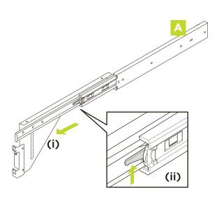
Separate each runner (A) into two parts by extending the guide (i) and pushing up on the lever (ii) while continuing to pull apart the two components. The guide should separate easily from the runner without too much force being applied.
