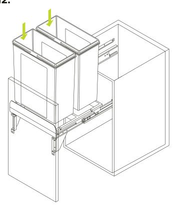
Place the bins into the frame to complete assembly. Note: Max weight capacity, including door if attached, is 25kg.
