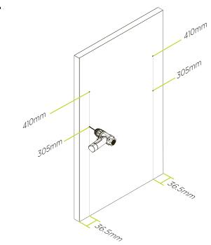
Measure from the bottom of door. Mark out and pre-drill four holes on the back of your cabinet door as pictured above. Use a 2mm drill bit to pre-drill holes to a depth of roughly 2.5mm.
