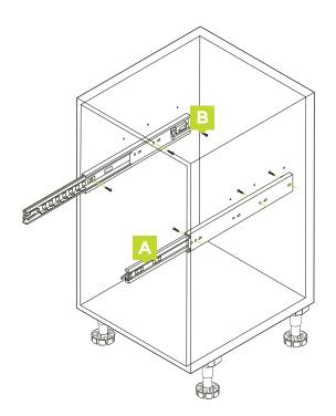
Using the lower sets of pre-drilled holes, align with the holes on the runners (A) and fix to the cabinet using  $6 \times 16$ mm wood screws (B) as pictured above.
