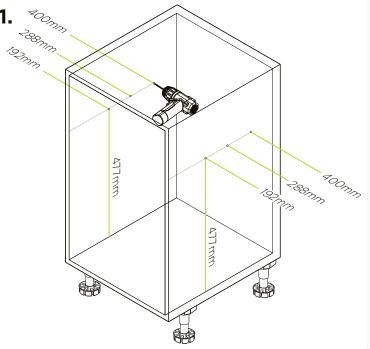
On both sides of your cabinet, draw a horizontal line 477mm up from the bottom. Measuring from the front of the cabinet along these lines, mark out the pre-drill holes at 192mm, 288mm and 400mm as pictured above. Use a 2mm drill bit to pre-drill holes to a depth of roughly 2.5mm.
