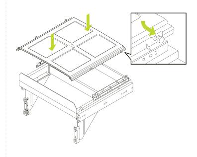
Slide the back plastic catches of the bin lid along the top of the lid brackets until both plastic catches fall into the channels at the back. The front two plastic catches should fit into the front channels at the same time.
