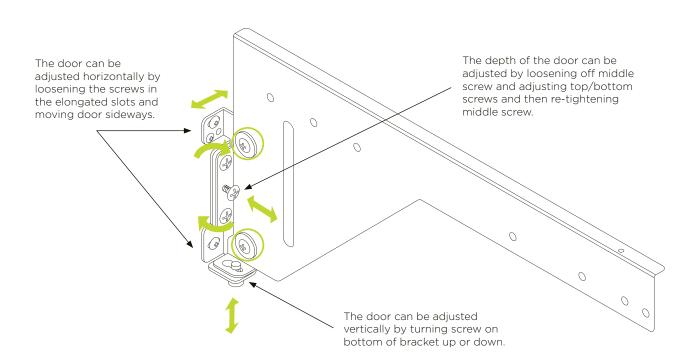
**Note:** Loosen off screws highlighted above before making any adjustments to the door. Once adjustments are completed, these screws must be tightened again.
