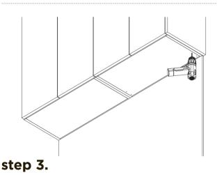
Using an 2.5mm drill bit pre-drill the marked out holes to a depth of 3mm
