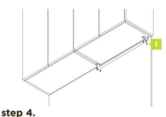
Align the assembled rail with the pre-drill holes and using the cabinet screws, fix the product to the cabinet.
