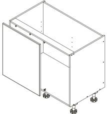
Attach the panel to cabinet making sure the marked line is even with the side of the cabinet.
