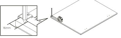
Mark a line 16mm all the way down the panel in from the side of the panel on the opposite end to the lugs.
