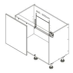
**Note:** To fit a larger door simply install the blind corner base panel further along the cabinet allowing the appropriate space to suit.
