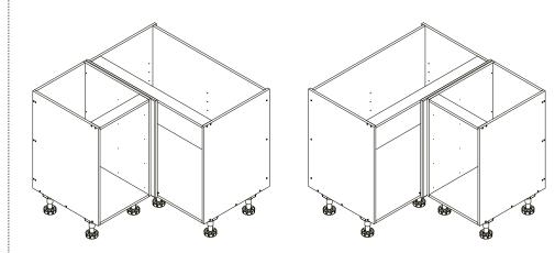
You can change the orientation of the cabinet for either Left or Right opening via the placement of the blind corner panel on to the cabinet. Consider the layout of your kitchen before installing the panel.
