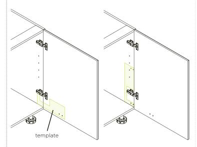
Use the template provided to mark out and pre-drill the holes for all three brackets. The placement of the template depends on which way your door opens.
