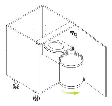
Swing the outer bucket towards the door and gently lift onto the door bracket. Once in place the bin should open and close automatically with the door.
