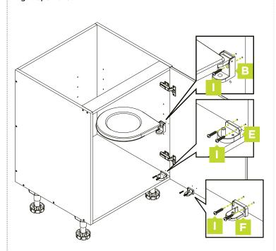
Using 6 of the screws (I) provided, fit the lid bracket (B), the outer bucket bracket (E) and door bracket (F) to the cabinet and door as pictured above.
