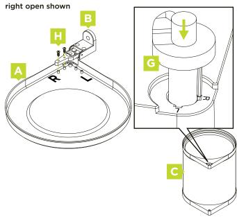
Fit the lid bracket (B) to the lid (A) using two of the screws (H) provided as pictured above. Ensure you have the correct orientation depending on which way your door opens. Fit the rotating axis (G) to the outer bucket (C), again ensuring you have the correct orientation.
