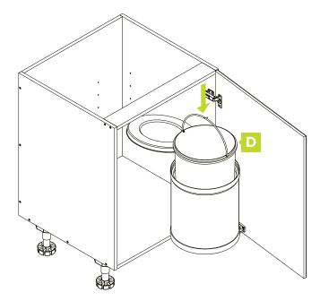
Place the bucket (D) into the outer bucket to complete installation.
