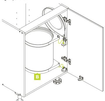
Fit the top of the outer bucket into the lid bracket ensuring that the bottom of the outer bucket fits over the pin on the door bracket, as pictured above.
