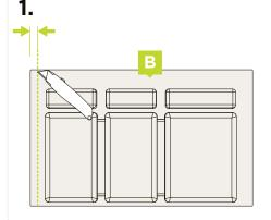
carefully trim the tray width at precut score line on underside of tray.
