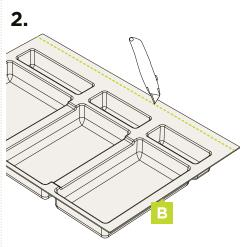
carefully trim the tray depth at precut score line on underside of tray.
