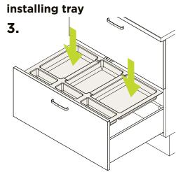
Install tray into the drawer. The tray is designed to be a tight fit. You can further trim the tray using a knife or by sanding edges as required.
