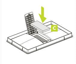
Open the flap on the underside of the bin lid and install the filter. Replace filter as needed.
