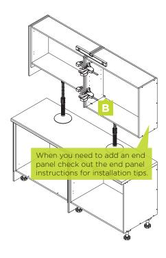
With the aid of cabinet supports, align cabinets and hold together using clamps.
