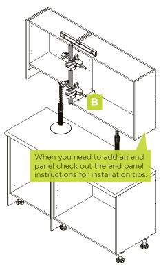
**Note:** AS/NZ Standards state the minimum clearance to the underside of the rangehood is 650mm from the trivet for gas and 600mm for electric cooktops or the appliance specification, whichever is greater. Be sure to check your appliance specifications before completing your installation.
