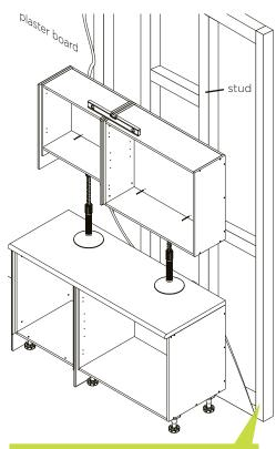
**Caution:** Please ensure all cabinets are screwed into your timber stud wall using a minimum of 65mm timber screws. If attaching to concrete, brick, steel or any other substrates seek advice from your hardware specialist.
