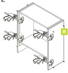
**Note:** end panels are only needed if you are using end panels either side of your oven cabinet. If you are not, move on to joining cabinets.
