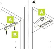
the push to release mechanism can be adjusted by turning the head of the mechanism clockwise or counter-clockwise.
