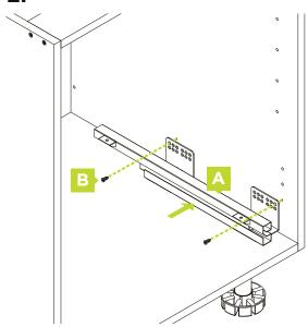
Align the runners (A) with the pre-drilled holes and using 4 x wood screws (B), fix the basket runners to the cabinet sides. Use a further 8 x 16mm wood screws to secure runners, ensuring the screws are spaced evenly on both runners and are mirrored from the left to right side.
