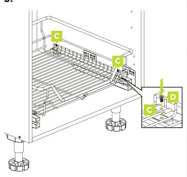
Place wire basket onto the runners, ensuring the metal supports are placed between the 2nd and 3rd wires at the front and back of the basket. Align the basket clips (C) and fix into place using the basket clip screws (D) and a hand held screw driver.
