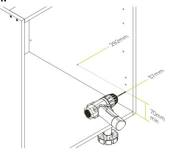
Calculate the desired height of your basket and runners. Mark out and pre-drill two holes on each side panel of the cabinet as pictured above. Use a 2mm drill bit to pre-drill holes to a depth of roughly 2.5mm. Note: Ensure the operation of the pullout basket will not be affected by any obstructions in the cabinet like hinges prior to pre-drilling holes.
