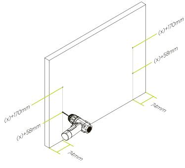
On the inside of your pot drawer panel, mark out and pre-drill four holes as per the diagram above, using measurements (x) from step 9. Use a 2mm drill bit to drill holes to a depth of roughly 2.5mm.
