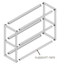
Note: If the frame is being installed underneath a wall cabinet or bulkhead, the top rails can be flipped upside down so that the shelf support can be screwed through as a fixing point.
