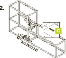
Use four 32mm tek screws provided to secure frames together. WARNING: Screws are provided to keep frames aligned and will not support significant weight. Be careful lifting and moving joined frames.
