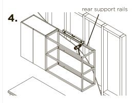
Sit the frame in position ensuring it is still square and level, and use the holes in the support rails to mark the wall.
