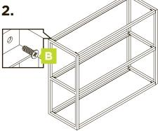
Use bolts provided to assemble the frame.
