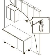
Use a stud finder to locate and mark the centre point of any stud that will be behind the frame. 2 studs are required to secure the frame, or one stud and a secure cabinet or wall to fix to sideways.
