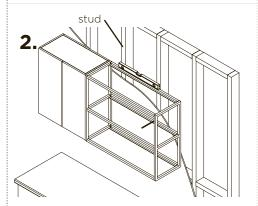
Use a stand or mounting rail to sit the frame in position and mark the location of the stud on all rear support rails.
