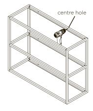
Use a 4.5mm HSS (steel drilling) drill bit to drill through the centre of each support rail in the marked locations of each stud.
