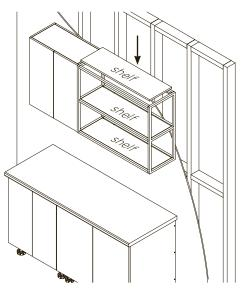
Screw the frame into the wall studs using the 70mm screws provided.
