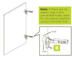
**Note**: install 2 more screws per carcase hinge plate (i.e.: a total of 4 screws) in round holes once the hinge has been adjusted!
