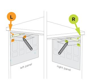
Use above template to mark drilling holes for lid brackets and drawer runner mounting position on left and right cabinet sides.
