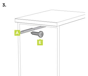
Attach both brackets uisng 4.5mm screws.
