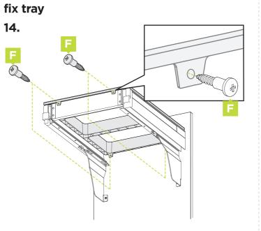
Fix tray to drawer assembly using 4 x 4.5mm stepped screws.
