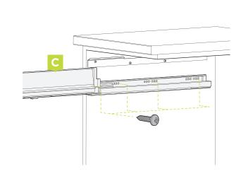
Mount metal sided drawer runners in marked positions below brackets using screws provided with runners.
