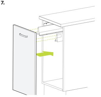
Mount drawer front brackets to rear of door. Clip brackets into place on metal sided drawer.
