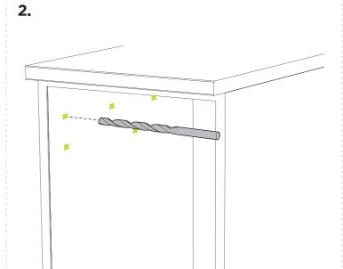
Pre-drill marked holes using 2.5mm drill bit. There will be 12 holes in total.
