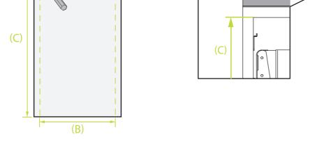
Measure the cabinet width (b), and the top inside cabinet height (c), mark on the door.
