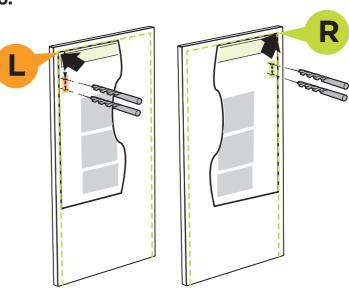
Align instructions and use side templates to mark front bracket positions. Once marked, pre-drill using 2.5mm drill bit.
