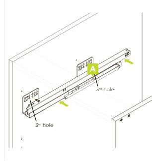
Using the top row of holes on the runners, screw the 3rd hole on the front set into the first pre-drilled hole on the cabinet. On the back set of holes screw the 3rd hole into the pre-drilled hole on the cabinet. Repeat for the other side.
