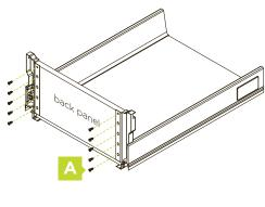
Fit the back panel into position, aligning the pre-drilled holes with the back bracket holes and screw into place using the 14mm screws.
