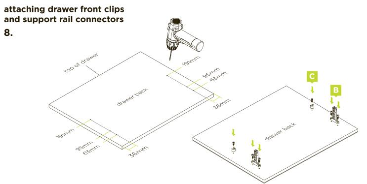
Draw a line 36mm in from each side of the drawer. From the bottom of the drawer mark a point 63mm, 95mm and 191mm on the lines.
