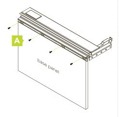
Slot the metal drawer side onto the base panel, aligning with the pre-drilled holes as pictured above.
