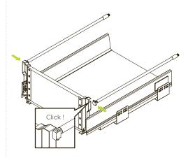
Push the end of the support rail onto each side of the back bracket of the drawer until it clicks into place.
