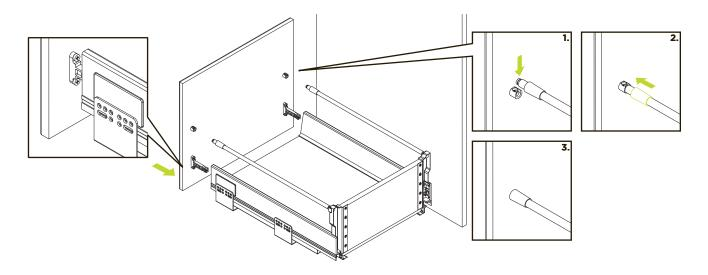
Align the drawer front clips with the drawer sides and push into place.
