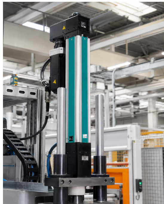
Figure 6: Example of a pressing station
