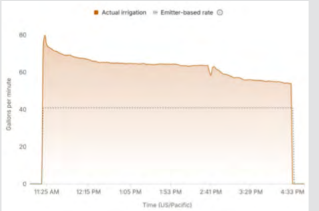
Irrigation monitoring equipment indicates higher than expected flow due to an issue with emitters.
