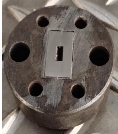
Corrosion nozzle with pair of small plates
