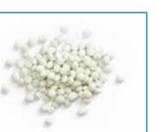
FED branch or for the pelletising of highly filled products with up to 70 % filling level (3). We use micropellets (4) for special processes, such as additive manufacturing, in order to ensure optimum intake be-haviour for small pelletising units. Long fibre pellets (5), made with the latest LFT technology allows us to produce rovings with very high strength products.
