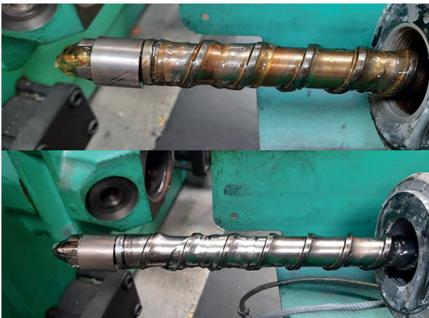
Screw build-up after processing polyketone, before and after purging with AF-Clean® for polyketone
