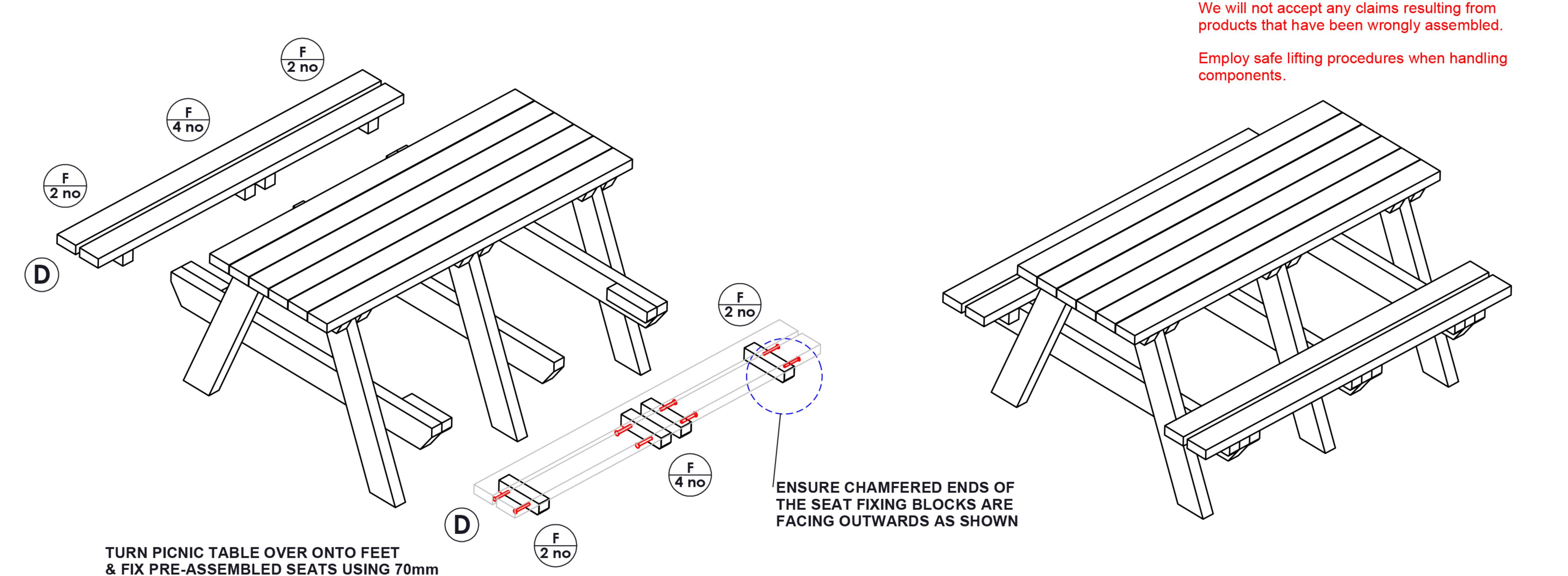
IMPORTANT - ENSURE THAT THE 16 no BRASS SEAT FIXING SCREWS ARE NOW FULLY TIGHTENED - THESE ARE SHOWN ON PAGE 1 OF 2
