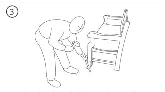
Insert drive bar through sleeve and into anchor. Position anchor through the strap.
