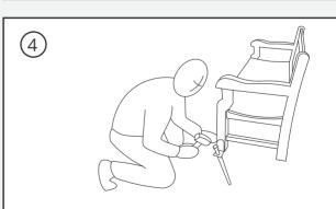
Remove sleeve and using the drive bar only, hammer down to drive out the anchor fluke.
