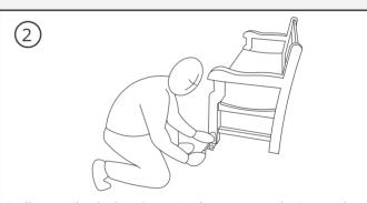
Drill two pilot holes, 3mm in diameter and 45 mm deep. Mark hole positions through the straps. Straps should be positioned on diagonally opposites
