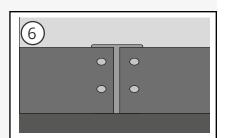
Where two strips meet, use a peg and scews to secure. Leave a 6mm gap between strips to allow room for expansion.
