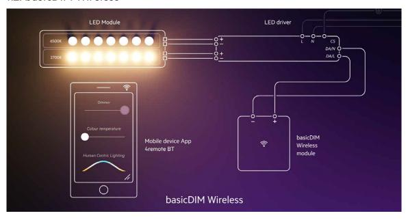
The wireless module does not need a control line. The light is controlled conveniently on a smartphone or tablet using the 4remote BT app.
