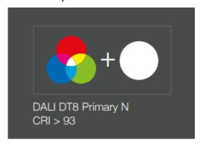
Primary N gives direct control over the light intensity of each available output channel.
