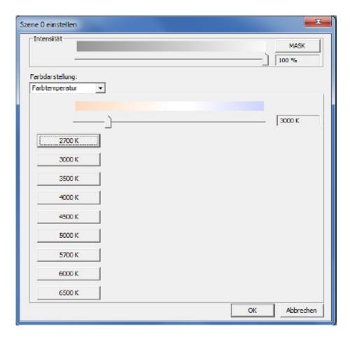
The SLE premium system can be adjusted via colour temperature and also via x-y coordinates.
