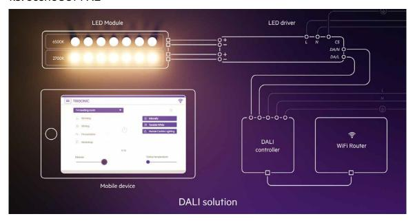
DALI systems like sceneCOM XL make it easy to implement and control complex lighting solutions. Built-in components can be controlled and adjusted directly.
