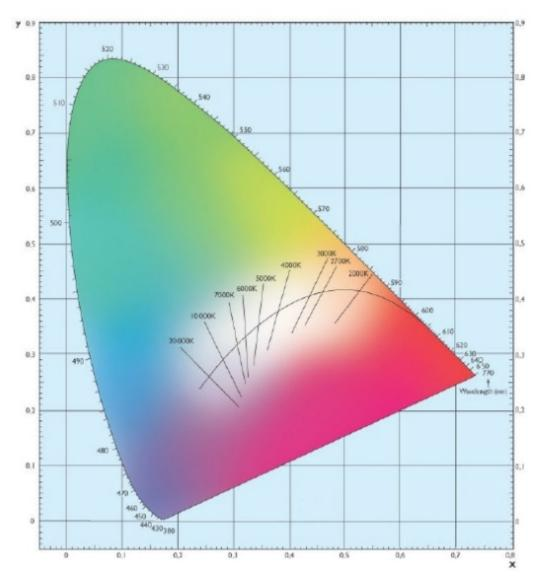
The output colour shall correspond as closely as possible to that shown in the figure for the point in the colour space defined by the x and y coordinates.
