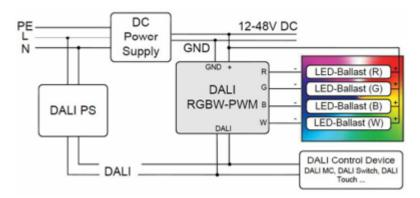
RGBWAF contains a method in which a minimum of 1 and a maximum of 6 output channels can be controlled independently of each other via "Arc Power Level".
