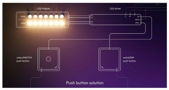
The combination of switchDIM and colourSWITCH buttons makes it easy to adjust the illuminance and colour temperature. The light can be dimmed using switchDIM, the proportion of cool white and warm white light can be mixed and customized with colourSWITCH.
