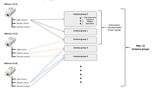
An instance is a "subcategory" of an input device. As an example, an MSensor V2 includes 3 of them: A **light sensor**, **motion sensor** and **remote control**.
