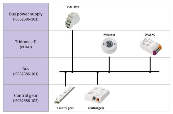
In the old DALI system, the commands from sensors and controllers (such as DALI XC) are processed directly by the control gear.
