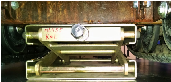
Elevate Trackchair with suitable lift or blocks, here you see the K&L model MC455 fat jack. (Purchase on-line.)
