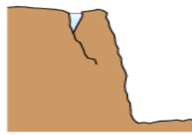
The temperature falls below 0°C. The water freezes and expands, making the crack bigger
