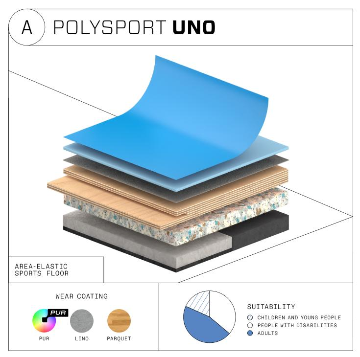
The area-reinforcing surface of POLY-SPORT UNO provides optimum stability for the athlete, enabling rapid reactions during team sports. Point loads on the surface are distributed across the surface area, meaning the system has high static and rolling load resistance for both sports equipment and tribunes. The
