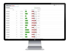
RailComm's iTrack solution is a real-time fully automatic railcar inventory system that allows yard personnel to identify and follow the location of every car and locomotive entering the facility. The solution integrates with the RailComm DOC Yard Automation system. Wheel sensors located at each switch turnout provide automatic and continuous tracking. As rail cars move through the yard, the system updates their location, which can be viewed from anywhere via a web-based interface.
