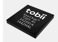
Tobii EyeChip is a custom designed highly optimized application-specific integrated circuit (ASIC), which contains Tobii's eye tracking algorithms
