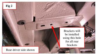
**Step 3:** Next obtain 1 of the short rear brackets. Take 10-24 x 1 ¼" bolt with a ¼" washer and place it through the very end hole of the bracket and screw on the jack nut (Collapsible insert) until snug with bracket. Now put the bracket up into the mounting hole as shown (Fig 2 & 3) with the bracket pushed up against the vehicle body and screw in place with #2 Phillips screw driver until fully tightened.
