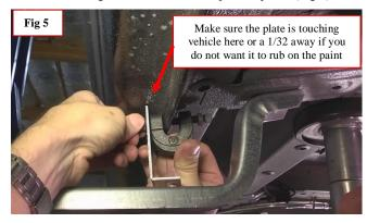
**Step 6:** Place a 5/16" bolt with washer through support plate and bracket. Then loosely secure with washer and serrated nut to hold in place. Only tighten nut until the head of bolt is through the nut. Repeat these steps for all rear brackets with the same mounting. (Fig 6)
