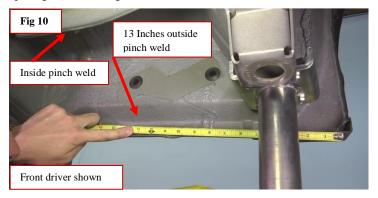
Step 11: Next we need to mark the inside pinch weld at 3 1/4". This is shown in (Fig 11) on the passenger side and is also indicated on the driver side picture in (Fig 10)
