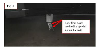
**Step 17:** Next adjust 100" board only to the end of the aluminum under the board to the edge of the last bracket on the back of vehicle.
