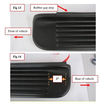
Step 14: This will show you the location and what the brackets should look like after you have them installed on the vehicle for the 100" board. The driver and passenger will look the same. If you are installing the shorter 39" board on the driver side you will only need the front 2 brackets installed.
