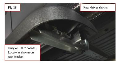
Step 18: Next tighten all fastens that were left loose to ad in board installation. Then make any adjustments up or down by loosening support plate bolt to adjust in slot. Once the boards are in place to your liking, tighten all fasteners on the boards and brackets. This will complete your installation. Enjoy!
