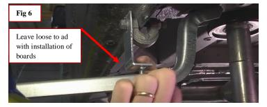
Step 7: Next install the middle bracket in front of the rear brackets just installed. Obtain one of the bolt plates and insert it into the hole as shown.
