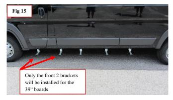
**Step 15:** Now install running boards on brackets. You may have different boards than shown. However, they will have the same type of mounting unless additional instructions are provided. Obtain the bracket to board bolt pack. Take out the provided 5/16"\*3/4" bolts. Slide the head of the bolts down the channels on the underside of the board. (Fig 15)
