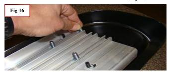
**Step 16:** Place the board on the installed mounting brackets. Align the bolts with the holes on the brackets and drop them into place. Next thread the provided 5/16" flange nuts loosely onto the bolts to secure brackets to the board
