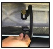
STEP 13 (Passenger Side): Attach two rear brackets to the passenger side. In the same manner as driver side brackets in steps 3-5.
