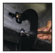
**STEP 6** (Drivers Side): **Avoid using power or air tools.** Tighten pinch weld mounts first then upper bolts. Tighten to 20ft lbs torque to secure the board to the truck.
