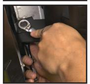
**STEP 16** (Passenger Side): Snug hardware for the first and second bracket. Tighten the bolt going up throught the pinch weld first to pull the board into place.
