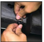
**STEP 4** (Drivers Side): Insert black head bolt and washer through pinch weld hole and secure with locking nut and washer.
