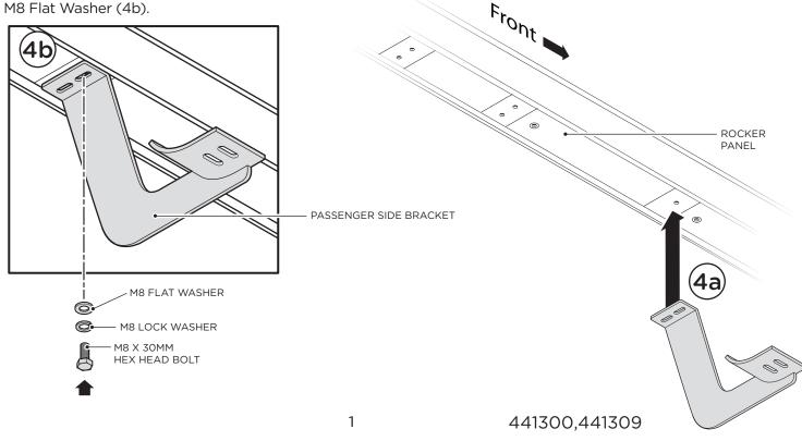
**5.** Position the remaining two (2) passenger side Brackets as shown (5a) and secure using two (2) M8 x 30mm Hex Bolts, two (2) M8 Lock Washers and two (2) M8 Flat Washers per Bracket (5b).
