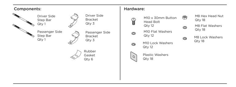
1. Remove all contents from the package and check stainless steel tubes for any damage. Also, verify that all components and hardware listed above are included before you begin installation.
