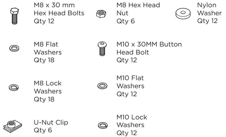
1. Remove all contents from the package and check stainless steel tubes for any damage. Also, verify that all components and hardware listed above are included before you begin installation.
