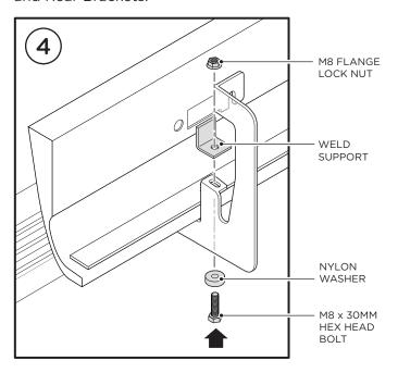
**5.** Complete the Front Bracket installation by fastening with one (1) M8 x 30MM Hex Head Bolt, one (1) M8 Lock Washer and one (1) M8 Flat Washer. Repeat for Center and Rear Brackets. Repeat these steps for driver side installation. When all hardware is in place, everything must be tightened. See Page 1 for Torque Specifications.
