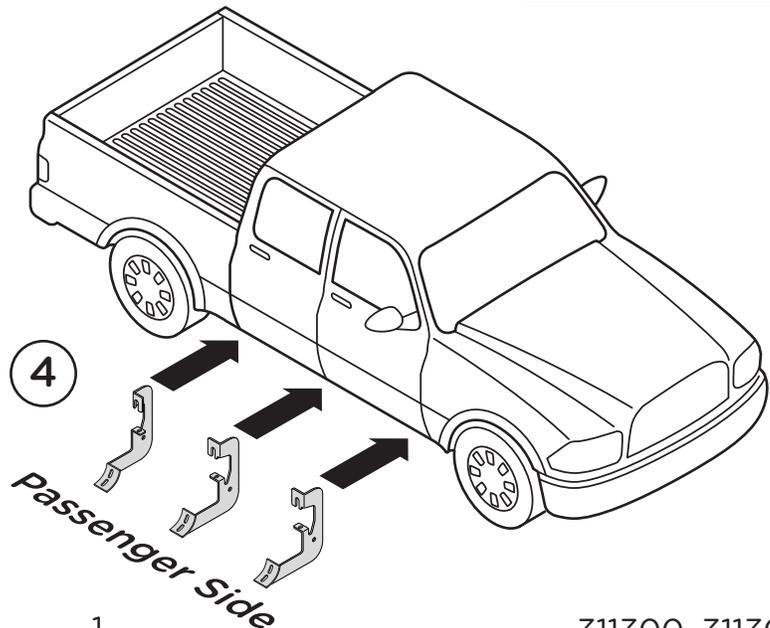
**5.** The Front & Center Bracket Step Bar Flange Cups face to the rear of the truck and the Rear Bracket Step Bar Flange Cups face to the front of the truck.
