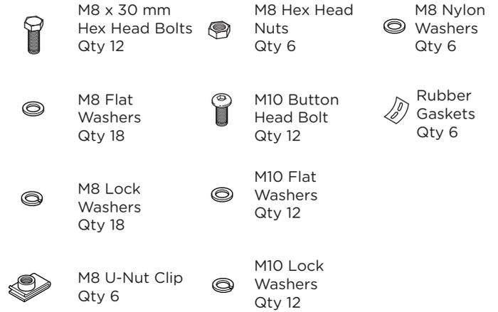
**1.** Remove all contents from the package and check stainless steel tubes for any damage. Also, verify that all components and hardware listed above are included before you begin installation.
