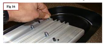
**Step 16:** Place the board on the installed mounting brackets. Align the bolts with the holes on the brackets and drop them into place. Next thread the provided 5/16" flange nuts loosely onto the bolts to secure brackets to the board
