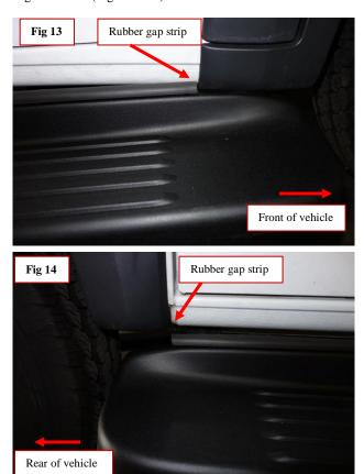
Step 14: This will show you the location and what the brackets should look like after you have them installed on the vehicle for the 84" board. The driver and passenger will look the same. If you are installing the shorter 39" boards you will only need the front 2 brackets installed.
