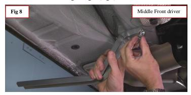
**Step 9:** Next install the tall support plate and clamp as was done for the rear brackets in (Fig 4, 5 & 6)
