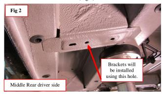
**Step 3:** Take 10-24 x 1 1/4" bolt with a 1/4" washer and place it through the very end hole of the bracket and screw on the jack nut (Collapsible insert) until snug with bracket. Now put the bracket up into the mounting hole as shown (Fig 2 & 3) with the bracket pushed up against the vehicle body screw in place with #2 Phillips screw driver until fully tightened. (Drill or small impact works best)
