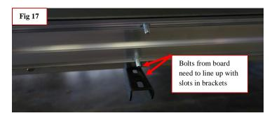
Step 17: Next adjust 84" board size only to the end of the aluminum under the board to the edge of the last bracket on the back of vehicle so the board fits flush with wheel well and is centered on vehicle.
