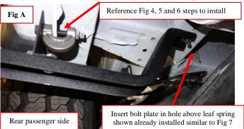
**Step 1:** The Middle Rear (Shortest) bracket will be installed on support gussets on each side of the vehicle. (Fig 2)
