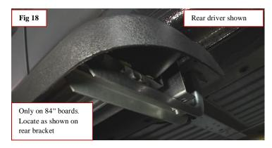
**Step 18:** Next tighten all fastens that were left loose to ad in board installation. Then make any adjustments up or down by loosening support plate 3/8" bolt to adjust in slot or move board in and out on bracket slots. Once the boards are in place to your liking, tighten all fasteners on the boards and brackets. This will complete your installation. Enjoy!
