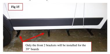
Step 15: Now install running boards on brackets. You may have different boards than shown. However, they will have the same type of mounting unless additional instructions are provided. Obtain the bracket to board bolt pack. Take out the provided 5/16"\*3/4" bolts. Slide the head of the bolts down the channels on the underside of the board. (Fig 15)
