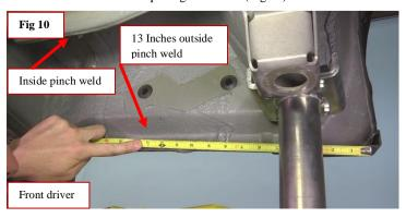
Step 11: Next we need to mark the inside pinch weld at 3 1/4". This is shown in (Fig 11) on the passenger side and is also indicated on the driver side picture in (Fig 10)
