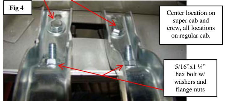
**Note:** For Super Cab and Super Crew mounting locations you will use a single bracket in the front and rear locations, **see figure 3**, on the center location it will look like **figure 4**. On the Regular Cab, both mounting locations will look like **figure 4**.
