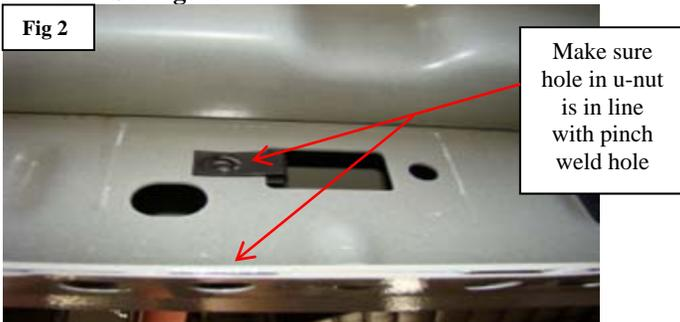
**Step 4:** Attach brackets to mounting locations using 5/16"x3/4" hex bolt and washer through bracket into previously installed u-nut and a 5/16"x1 1/4" hex bolt, washers and nut through the pinch weld and bracket. **See figures 3&4.**
