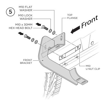
**6.** Complete the installation of the Front Bracket by using two (2) M10 Hex Head Nuts, four (4) M10 Flat Washers and two (2) M10 Flat Washers. Repeat this process for the Rear Bracket. Hand tighten all hardware.
