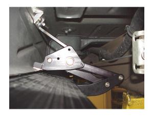
13. Install idler linkage assembly onto rear of vehicle using 0.08" spacer between mount and sheet metal
