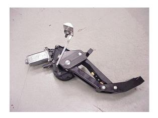
9. Install upper sill mount and bracket onto driving linkage assembly
