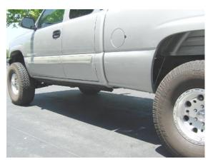
With the running board in the retracted position under the sill it does not interfere with the body lines of the truck and is virtually unnoticeable. With the new kinematics of the linkage assembly the deployment time of the step is under 1 second.
