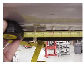
6. Locate rear hole on drill jig at measured distance
