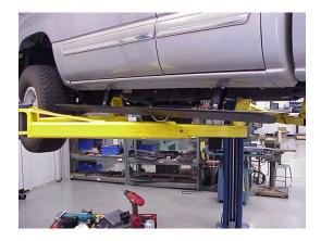
14. With board deployed in a horizontal position tighten bolts on both upper mounts
