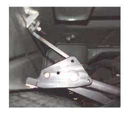
15. Make sure board does not hit sill or hardware in retracted position, adjust if necessary
