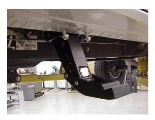
10. Install driving linkage assembly vehicle using front holes drilled into sheet metal.
