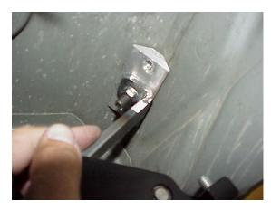
11. Locate mounting position of upper sill mount and drill two 316" holes12. Use self tapping sheet metal screws to
