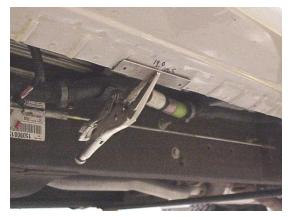
2. Locate front hole on drill jig at measured distance and secure jig to sheet metal
