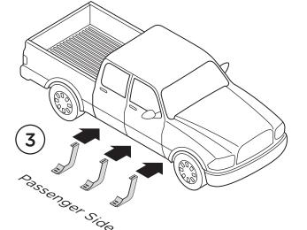
**4.** All passenger side Brackets are identical with the bracket cradle facing toward the rear of the vehicle. Install the first passenger side Bracket closest to the front wheel. Align with existing factory holes in the rocker panel as shown (4a), Secure the first Bracket using one (1) M8 x 30mm Hex Bolt, one (1) M8 Lock Washer and one (1) M8 Flat Washer (4b).
