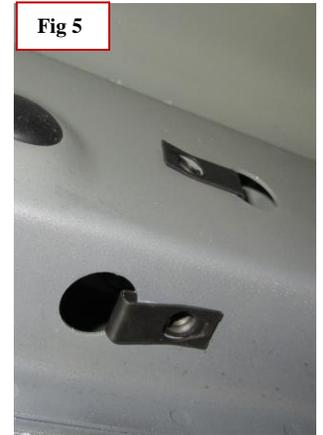
**Step 4:** Please use (Fig 1 & 2) for reference. Starting on the driver side front location use bracket shown (Driver Front/Passenger Rear). This bracket will be used on the first 3 bracket locations on the driver side. The very rear bracket towards the bed will use the bracket shown (Passenger Front/Driver Rear). Install using 5/16" bolts with washers. (Fig 6)
