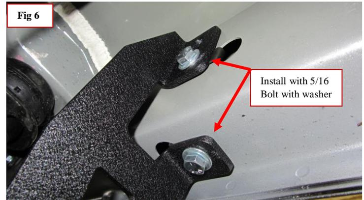
**Step 5:** Now with everything installed. Take a look at the board on your vehicle. There is a lot of adjustment in the kit to get the board where you like them. Adjust boards in and out and side to side with the slots on the bracket where board mounts. Adjust the front and rear brackets first and finish with the middle. Once the boards are in place to your liking, tighten all fasteners on the boards and brackets. This will complete your installation. Enjoy!
