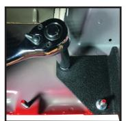
**STEP 6** (Drivers Side): **Avoid using power or air tools.** Tighten to 20ft lbs torque to secure the board to the truck.
